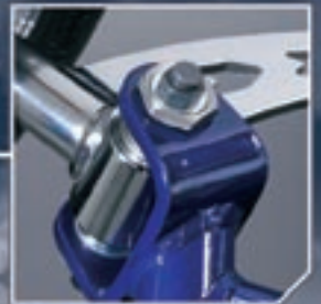
Adjustable camber/caster, Ackerman and front ride height
