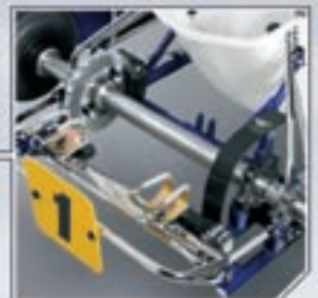
Adjustable/removable rear torsion bar
