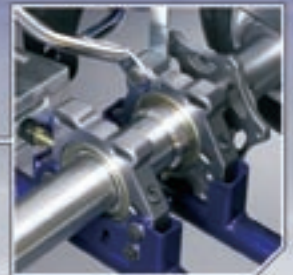
Unique full-height one-piece machined billet alloy bearing flanges
