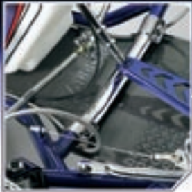
Adjustable/removable front torsion bar & carbon fibre laminate floortray
