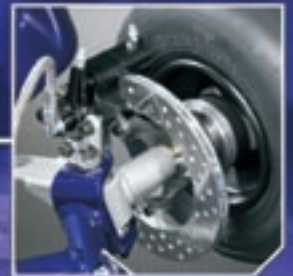
Unique Arrow ventilated front brake discs
