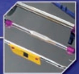
Adjustable/removable rear torsion bar
