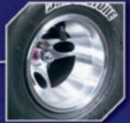
One-piece machined alloy 3-spoke wheels
