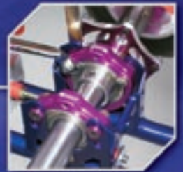
Rear axle supported by three bearings
