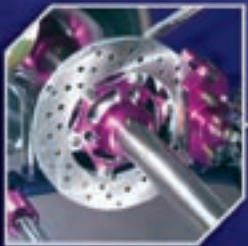
Ventilated 18mm wide brake disc & machined billet alloy 2-spot caliper
