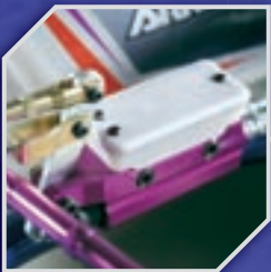
Machined billet alloy brake master cylinder
