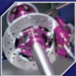
Optional Ventilated 18mm wide brake disc & machined billet alloy 4-spot caliper
