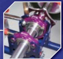
Rear axle supported by three bearings
