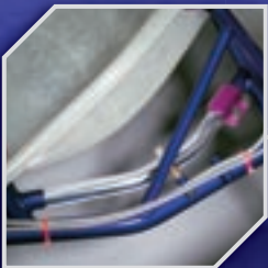
Removable side torsion bar
