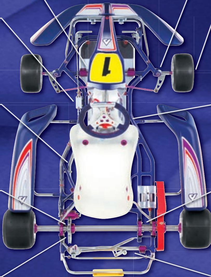
Standard Ventilated 18mm wide brake disc & machined billet alloy 2-spot caliper
