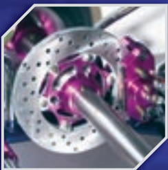
Standard Ventilated 18mm wide brake disc & machined billet alloy 2-spot caliper
