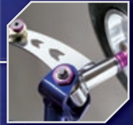
Adjustable camber/caster and front ride height
