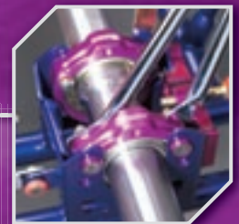
50mm axle supported by three bearings
