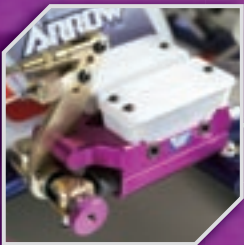
Twin machined billet alloy master cylinders
